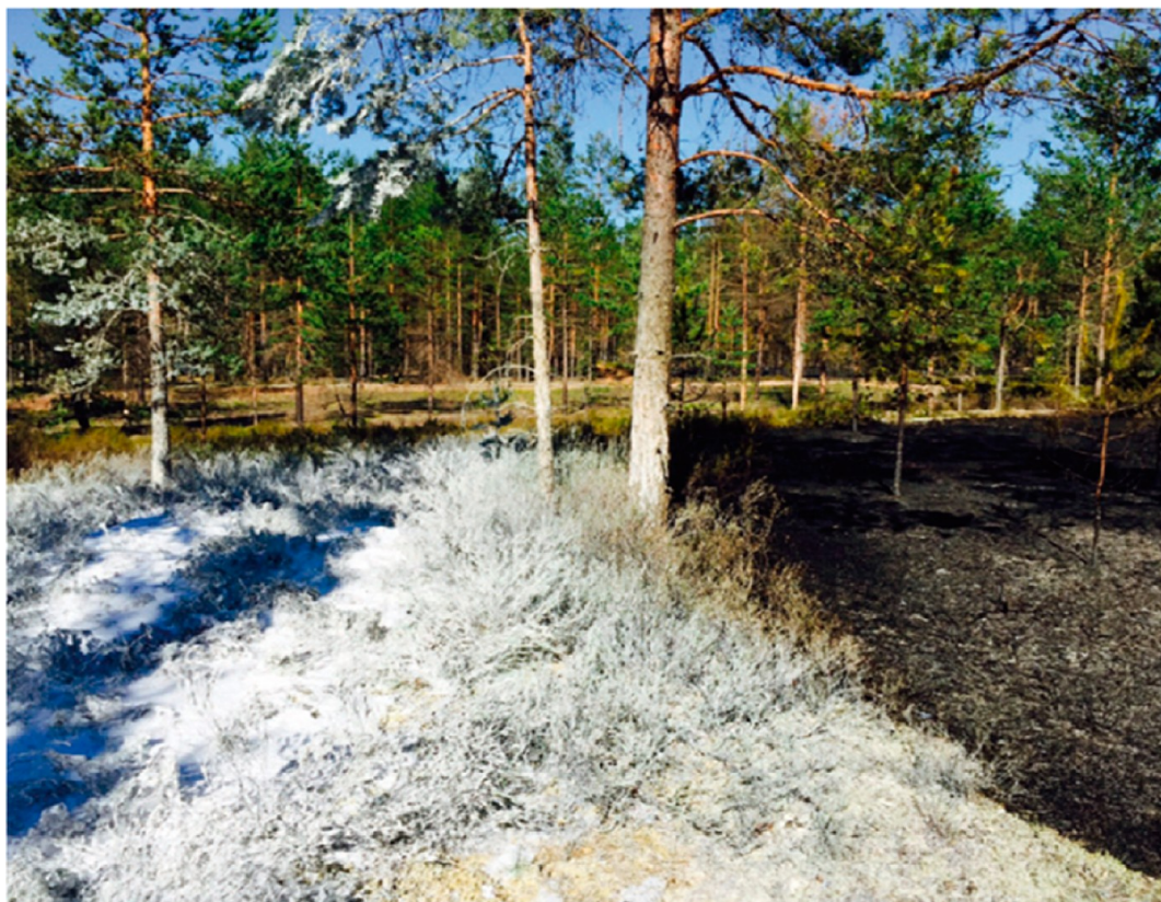
Figure 9. Complete cessation of fire spread upon the contact with a silica-based foam fire retardant belt after 2 d. Self-hardening silica-based foam was generated via FHF-30 extinguisher and contains 6% SDS, 30% pure \text{SiO}_2 , and 64% \text{H}_2\text{O} . The estimated foam multiplicity is 20. The square 500 \text{m}^2 were treated with consumption index 1.06 \text{L}/\text{m}^2 . The full demonstration available here https://www.youtube.com/watch?v=kWKB0r4i2Hk .
