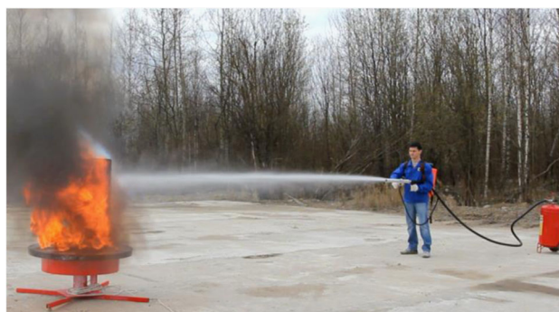
Fig. 5 Fire-extinguishing process of the model fire seat (class A)
