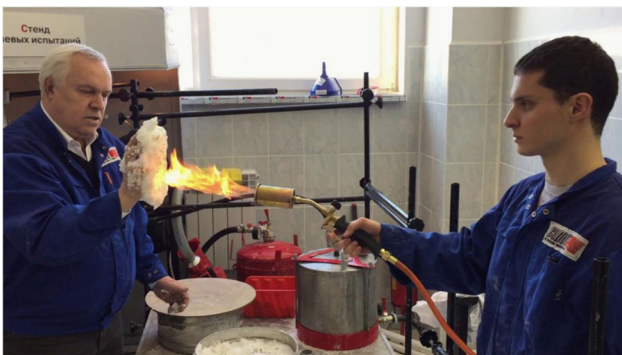
Fig. 1 Opened fire source exposure on the fragment of FHF
