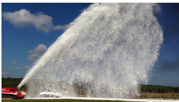
Fig. 8 FHF delivery by fire-fighting tracked vehicle “Yamal-201”
