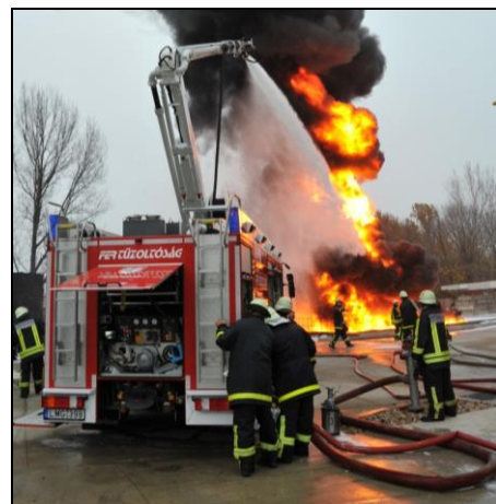
HydroChem monitor mounted on extinguishing boom (Photo: FER Százhalombatta)
