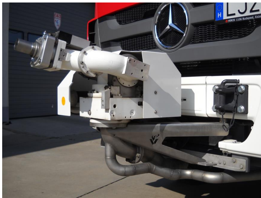
Vogt HydroChem Monitor (Photo: FER Algyő)
