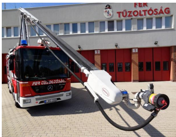
HydroChem monitor mounted on extinguishing boom (Photo: FER Százhalombatta)
