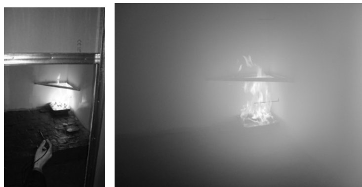
Fig. 3. Images taken during tests. From left to right: Ethanol pan fire before the water mist discharge, and during the water mist discharge.
