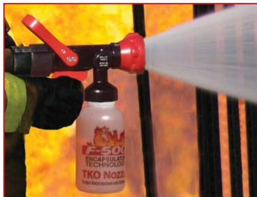
Fast response is delivered by the pistol grip, F-500 EA Turbo Knockdown and Overhaul (TKO) Nozzle. The nozzle carries two quarts of F-500 Encapsulator Agent, which instantly educts a pre-set percentage of solution into the water stream (0.5%, 1% or 3%). Six bottles of F-500 EA are provided with the FRMU for replacement in seconds during a fire or spill, although a portion of a single
