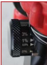
bottle has been shown to be sufficient to extinguish a car fire. The TKO Nozzle can reach about 28 feet with a streaming pattern and quickly adjust to a conical pattern. The F-500 EA TKO Nozzle greatly reduces steam, smoke and toxins, while using less water and very little agent.
