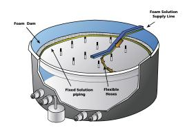
Fig 8.6 – Catenary System Protection of Open Top Floating Roof Tanks
