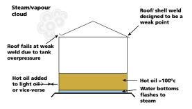
*Fig 2.13 Tank roof separating due to internal pressure rise*
