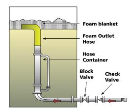
Fig 8.3 – (b) Semi-subsurface protection system. During discharge
