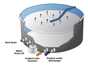
Fig 2.9 - Example of Open Top Floating Roof Tank
