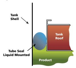
Fig 2.11 - Flexible resilient tube type seal
