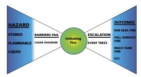
Fig 5.1–'Bow Tie Diagram' Showing Failure of Barriers
