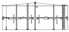
Fig 2.8 - Example of internal floating roof tank
