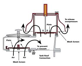
Fig 2.5 -Typical example of a Pressure/Vacuum Valve on fixed roof tanks
