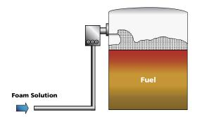
Fig 8.1 – Top Pourer Foam Application to Storage Tank
