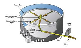
Fig 8.7 – "Coflexip" System Protection of Open Top Floating Roof Tanks
