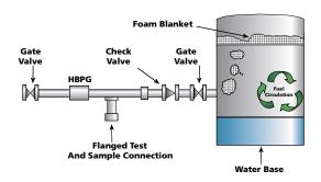
Fig 8.4 – Subsurface Protection of Cone Roof Storage Tanks
