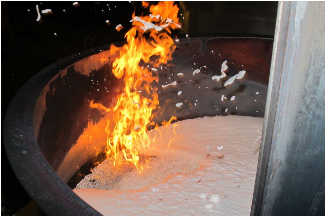
Figure 57 Test #13 (043) The layer of cellular glass is nearly covered by the foam and the remaining fire is almost extinguished.
