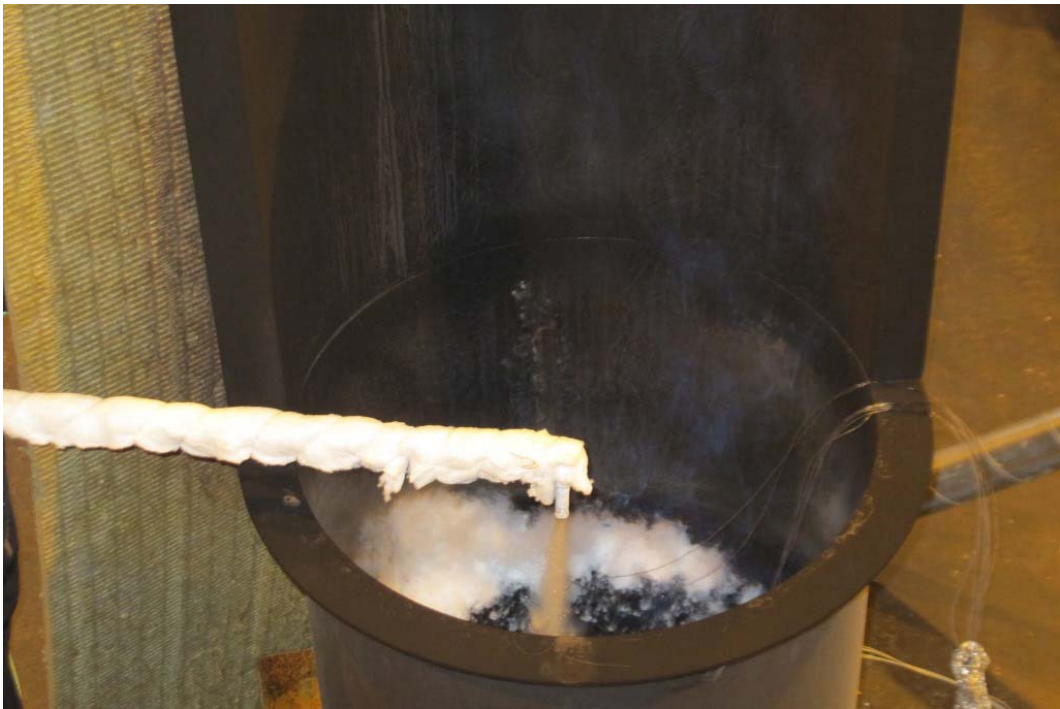
Figure 29 Test#22 (032) Liquid nitrogen controlling the fire but blue, almost invisible flames, are still present.
