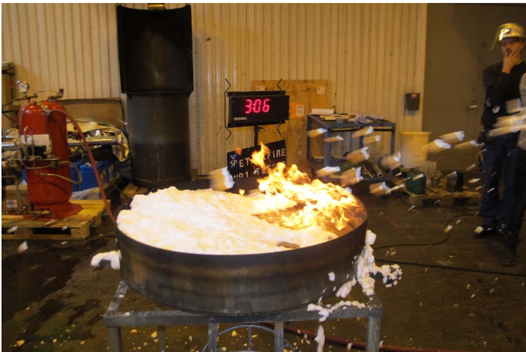
Figure 38 Test#28 (032) Test in the 2580-tray using CAF and Type III foam application. Although a significant portion of the foam landed outside the fire tray due to bad coherence of the foam stream, an effective foam layer was established on the fuel.
