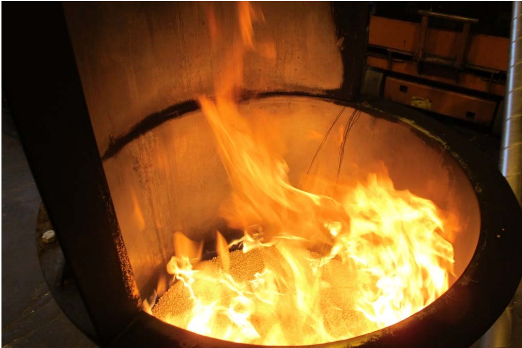
Figure 31 Test #23 (054) The fire intensity is reduced by the layer of cellular glass.
