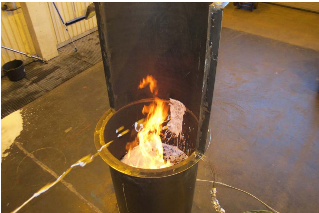
Figure 5 Test#5 (005) 450 mm fuel, preburn 2 minutes, foam impact position 0,35 m above fuel surface.
