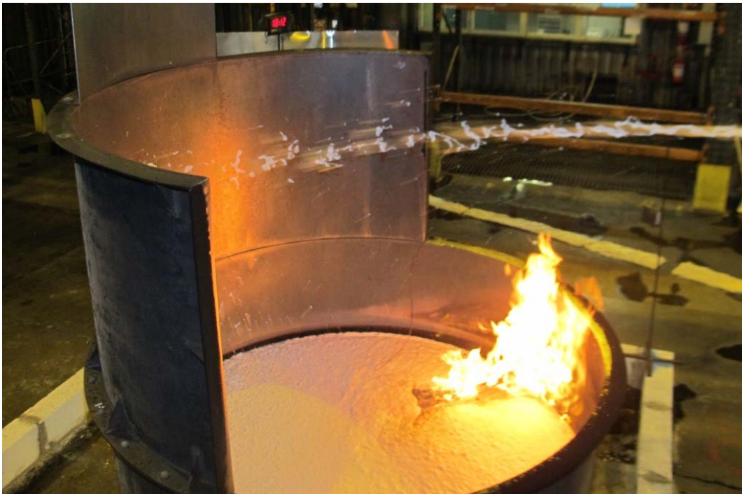
Figure 53 WP2-Test #12 (012) Similar to WP2-Test#5 ( 3,63 \text{ l/m}^2 \text{ min} ) but using the F3 foam at 6%.
