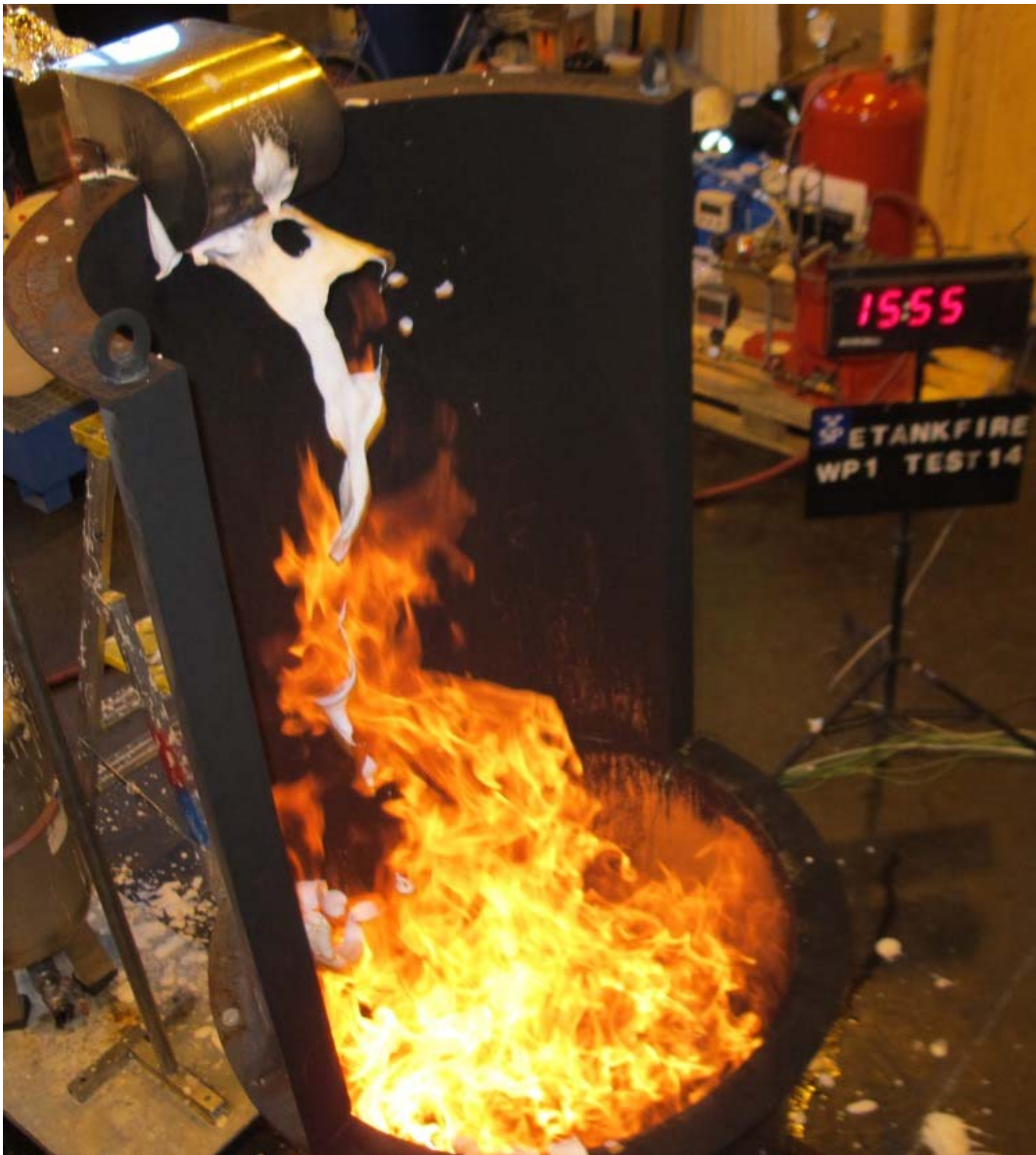
Figure 16 Test#14 (012) CAF application via the foam chamber after 15 min. Free fall of foam due to the hot steel wall (0:55 min:s after start of application).
