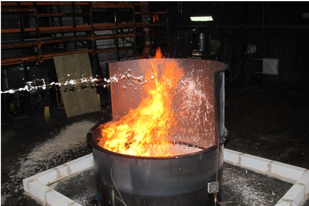
Figure 43 WP2-Test#3 (035) Similar to WP2-Test #2 but using lower application rate (4,77 l/m 2 min)
