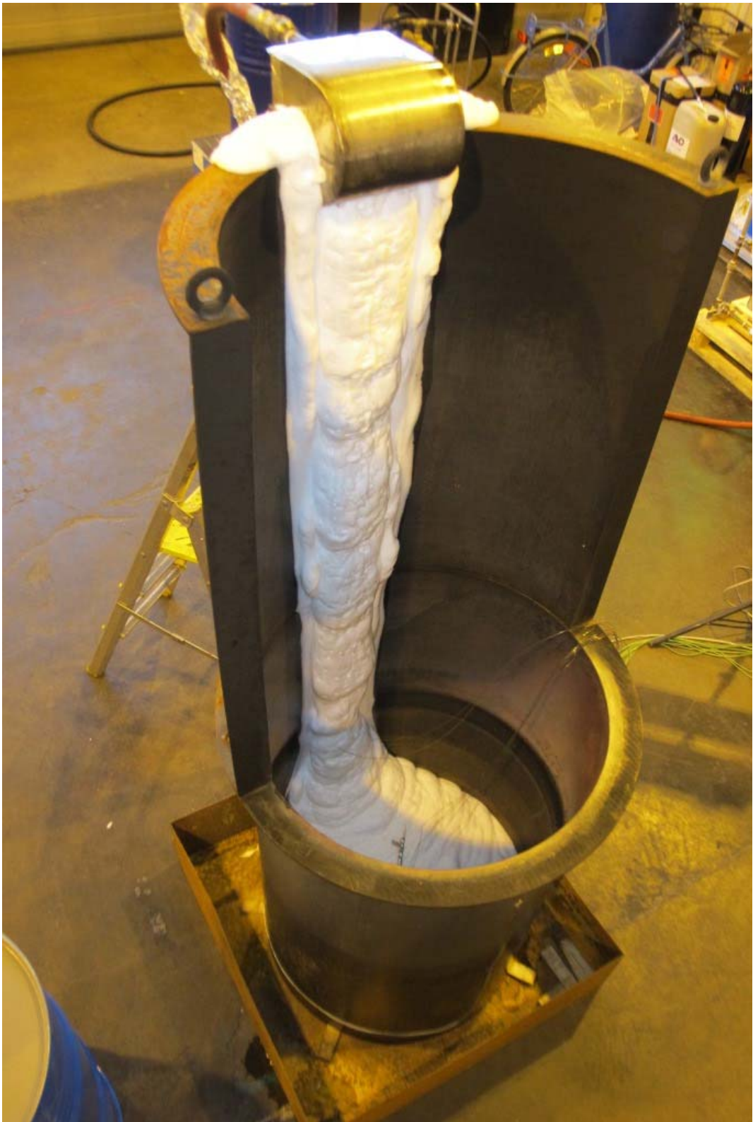
Figure 15 Test#14 (008) CAF application via the foam chamber on a cold steel surface.
