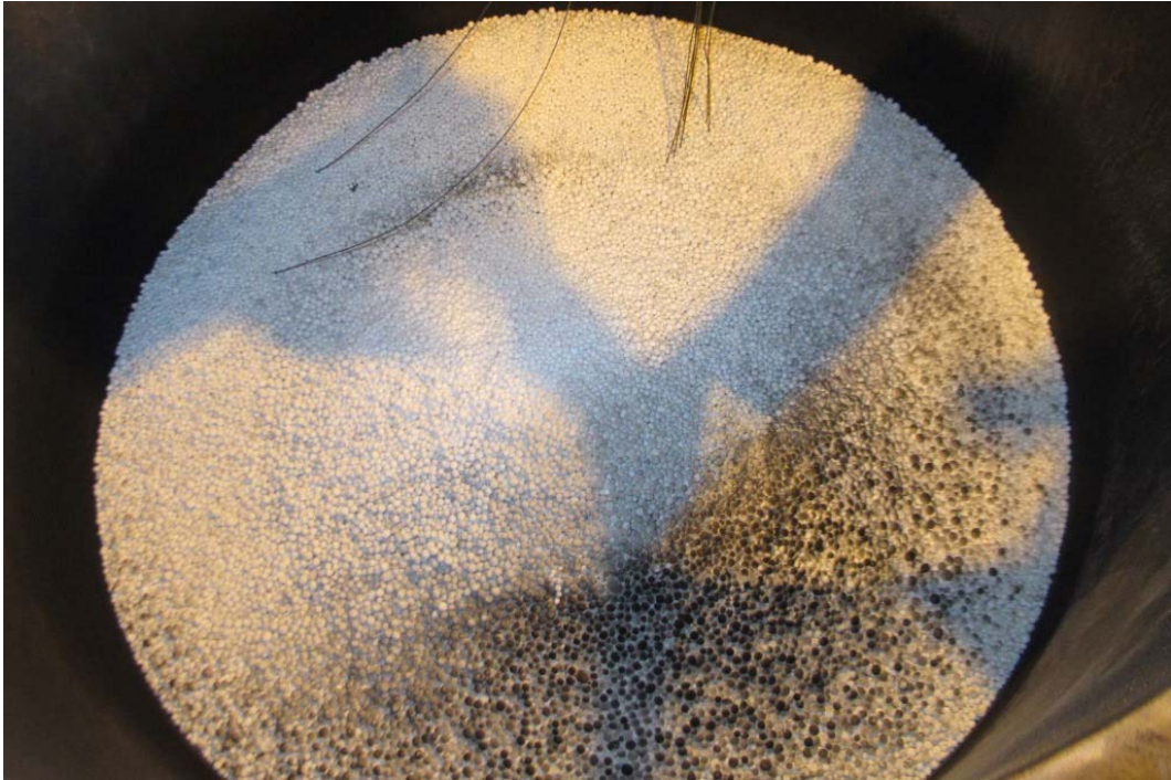
Figure 33 Test#23 (061) The layer of cellular glass after the fire has been manually extinguished. It was observed that there was a considerable difference in the depth of the cellular glass layer and the black surface indicate the area with the least depth.
