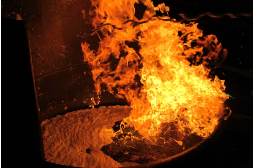
Figure 52 WP2-Test #11 (074) Similar to WP2-Test #9 ( 3,63 \text{ l/m}^2 \text{ min} ) but using F3 foam at 3%.
