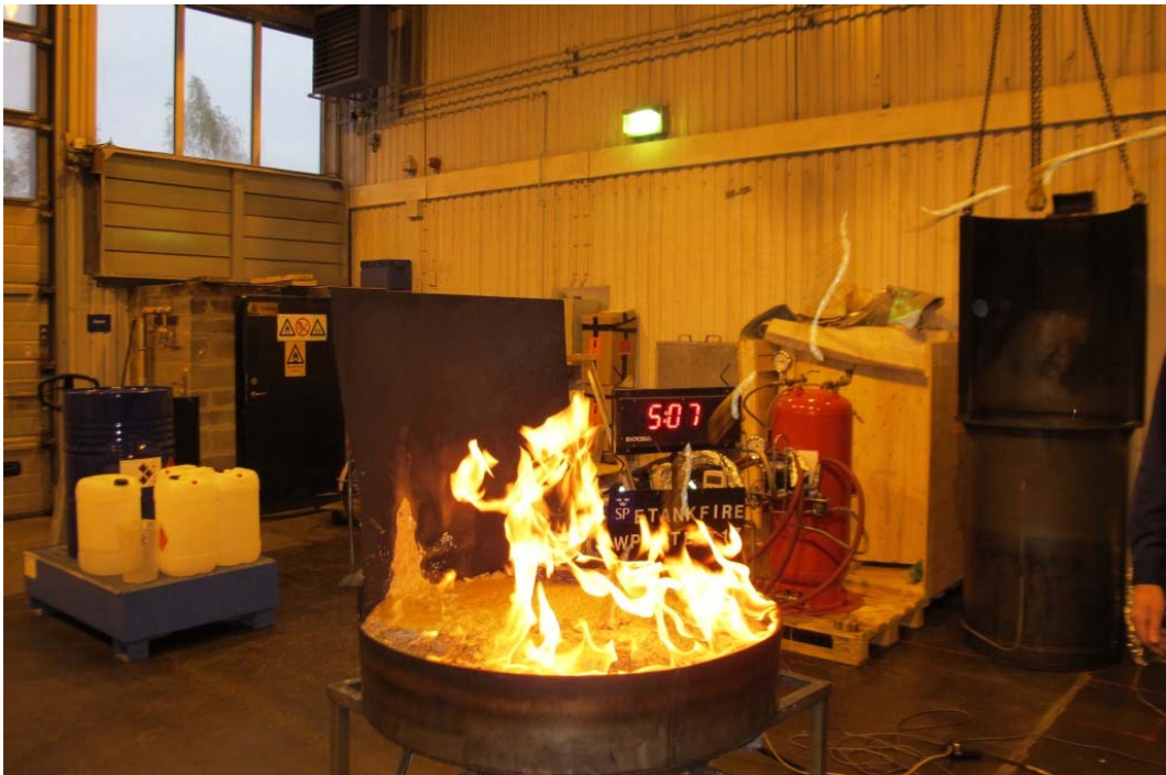
Figure 20 Test#17 (006) Test in the 2580 tray using AVD and a UNI86R nozzle.
