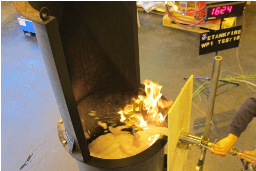
Figure 22 Test#18 (025) Planned to be similar to test 10 but using F3 foam. Bad coherence of the foam stream resulted in a mixture of Type II and Type III application.
