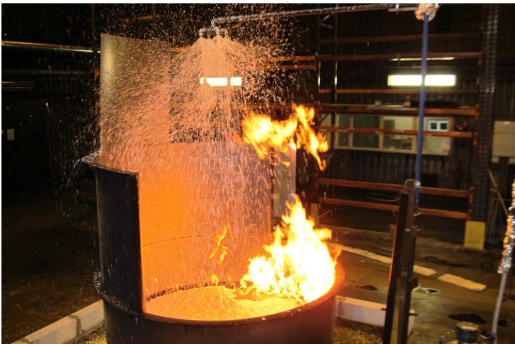
Figure 51 WP2-Test #10 (034) Type III application of CAF (AFFF-AR 6%, 3,63 l/m 2 min) using a “spiral jet nozzle” arrangement located 2,55 m above the fuel surface .
