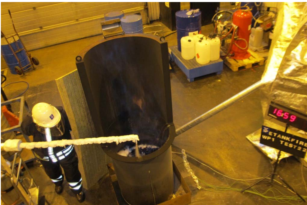
Figure 28 Test#22 (031) Liquid nitrogen applied directly onto the burning fuel surface.
