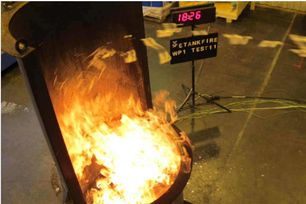
Figure 12 Test #11 (005) Foam impact position 1,05m above fuel surface but changed every 3 minutes (picture show foam impact on the right hand side).
