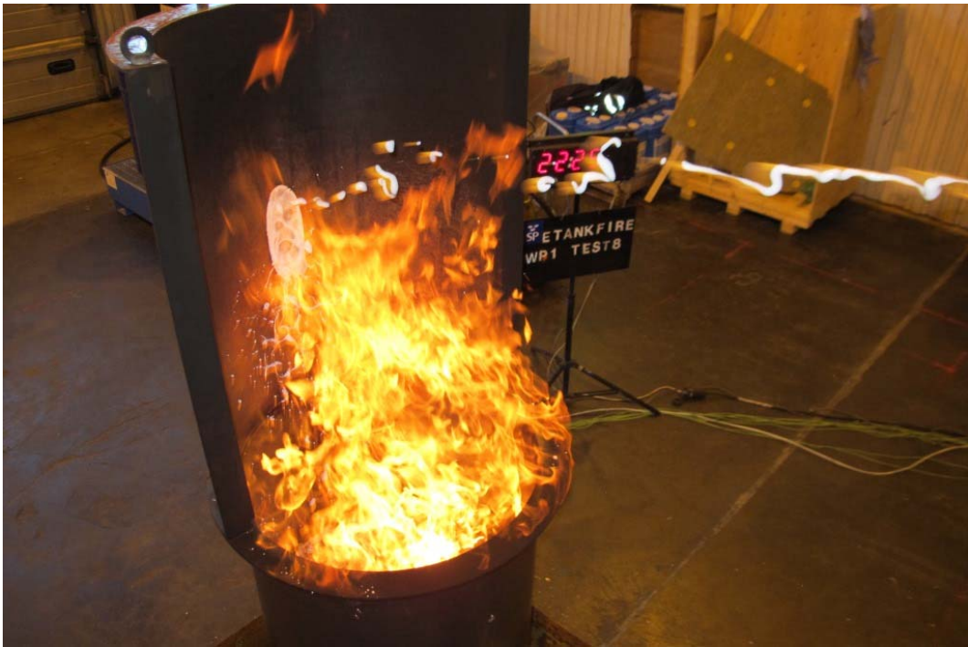
Figure 8 Test#8 (009) Foam impact position higher, 1,05m above fuel surface.
