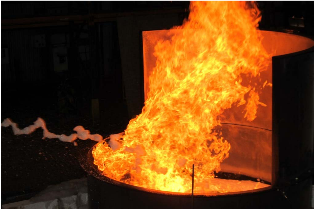
Figure 44 WP2-Test #4 (023) Type III application of medium expansion foam (MEX), nozzle position 1,05 m above the fuel surface. ( 4,77 \text{ l/m}^2 \text{ min} )
