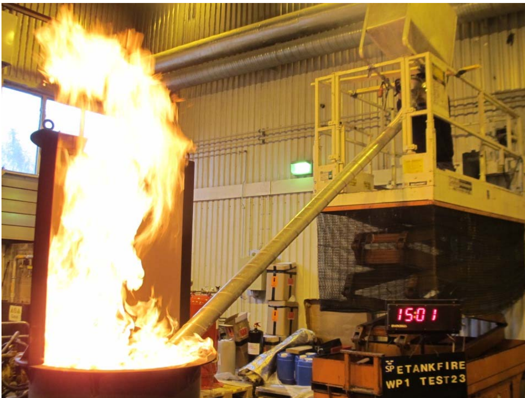
Figure 30 Test#23 (044) Application of cellular glass corresponding to an average thickness of 183 mm.
