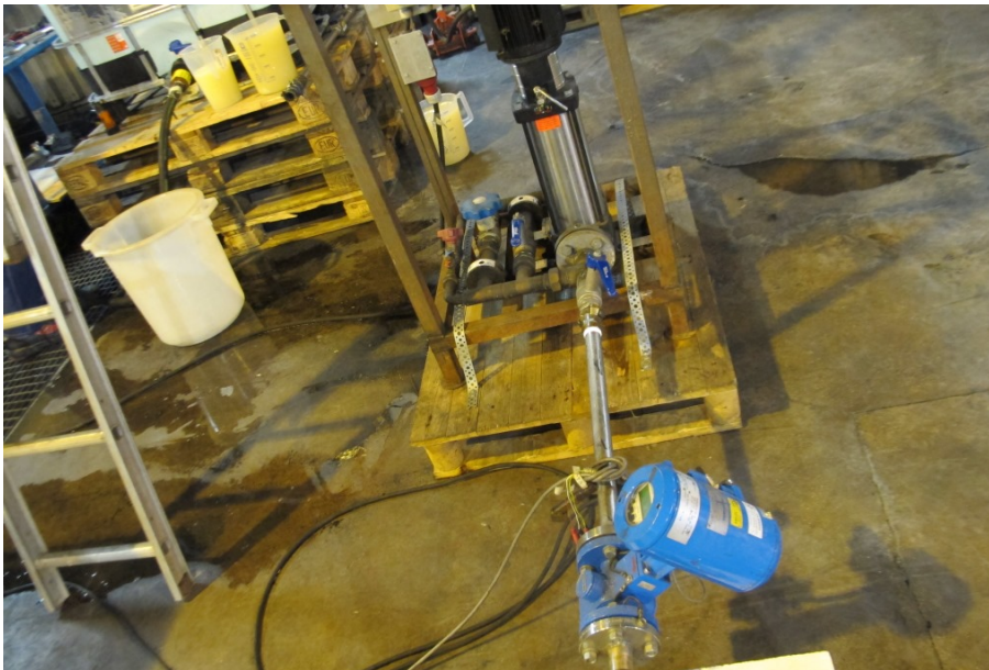
Figure 10 Foam supply equipment used during the WP2 tests. The IBC (partly visible upper left) was used to hold the premix solution and was connected to a centrifugal pump followed by a flow meter. The pump had a by-pass arrangement between the pressure and suction side, to allow a fine tuning of the delivered pressure and flowrate to the foam nozzle.
