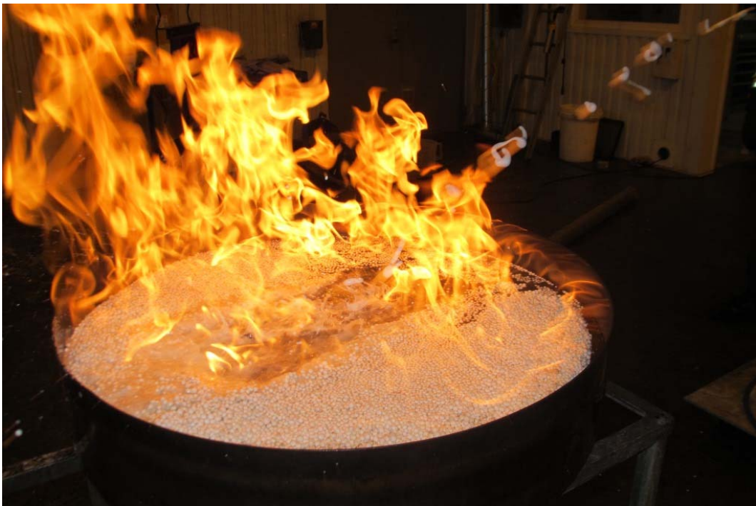
Figure 36 Test#26 (011) Test in the 2580-tray applying cellular glass (average 10 mm) followed by Type III foam application. The cellular glass layer was too thin and was pushed away by the foam stream at the point of impact.
