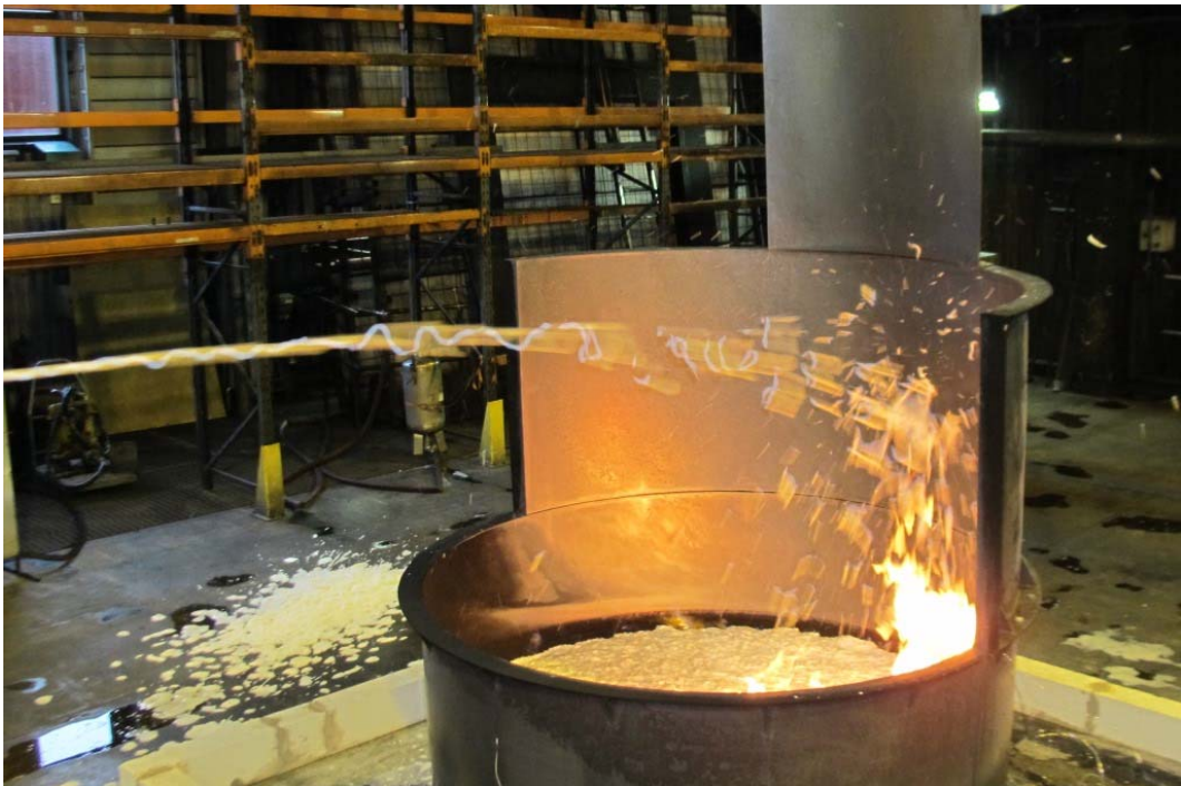
Figure 49 WP2-Test #9 (016) Similar to WP2-Test#5 (AFFF-AR 6%, 3,63 l/m 2 min) but applied as CAF.
