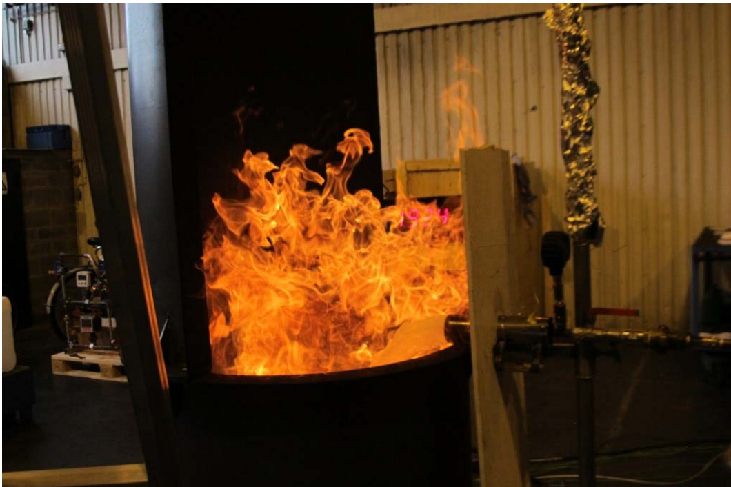
Figure 11 Test#10 (065) Medium expansion foam, Type III application 0,55m above fuel surface.
