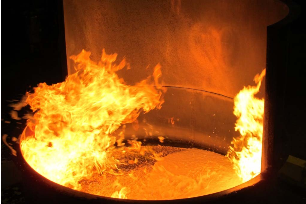
Figure 56 WP2-Test #13 (041) Type III foam application starts 10 min after application of cellular glass. A foam layer is immediately established on the cellular glass.
