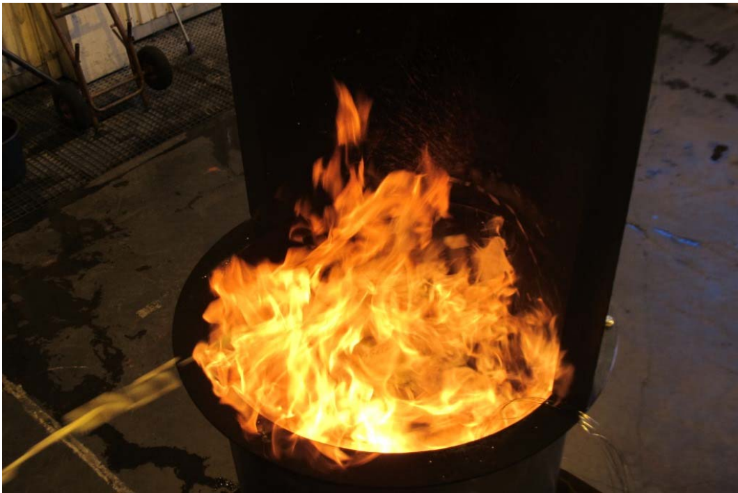
Figure 6 Test#6 (013) 450 mm fuel, preburn 10 minutes, foam impact position 0,35 m above fuel surface.
