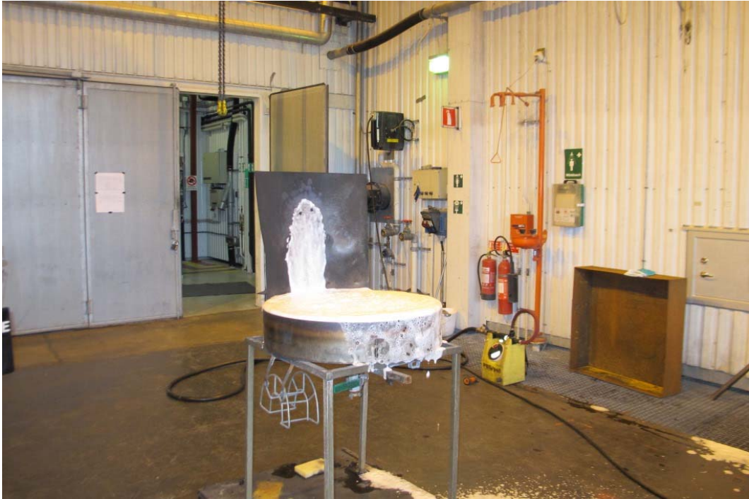
Figure 2 Test#1 (032) Picture after extinguishment showing the foam impact point at the backboard.
