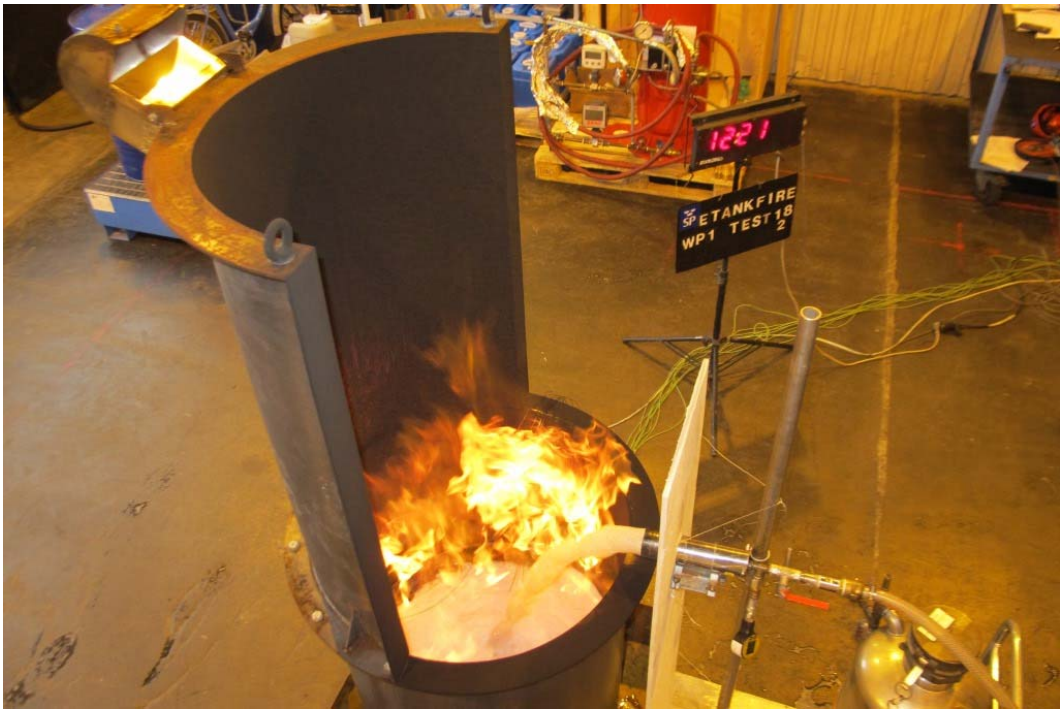
Figure 23 Test#18B (031) Repeat of Test # 18 with improved coherence of the foam stream resulting in a Type III application. (Fuel from Test #18 re-used and preburn time 10 minutes.)
