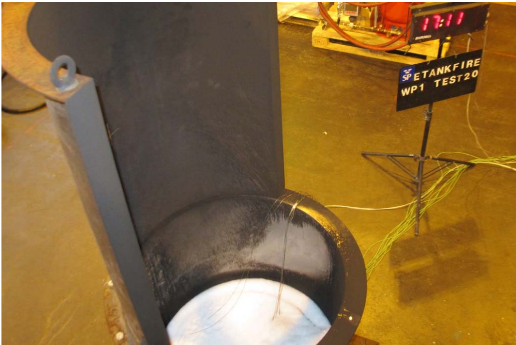
Figure 25 Test#20 (009) Similar to Test #8 but using AFFF-AR at 6%.
