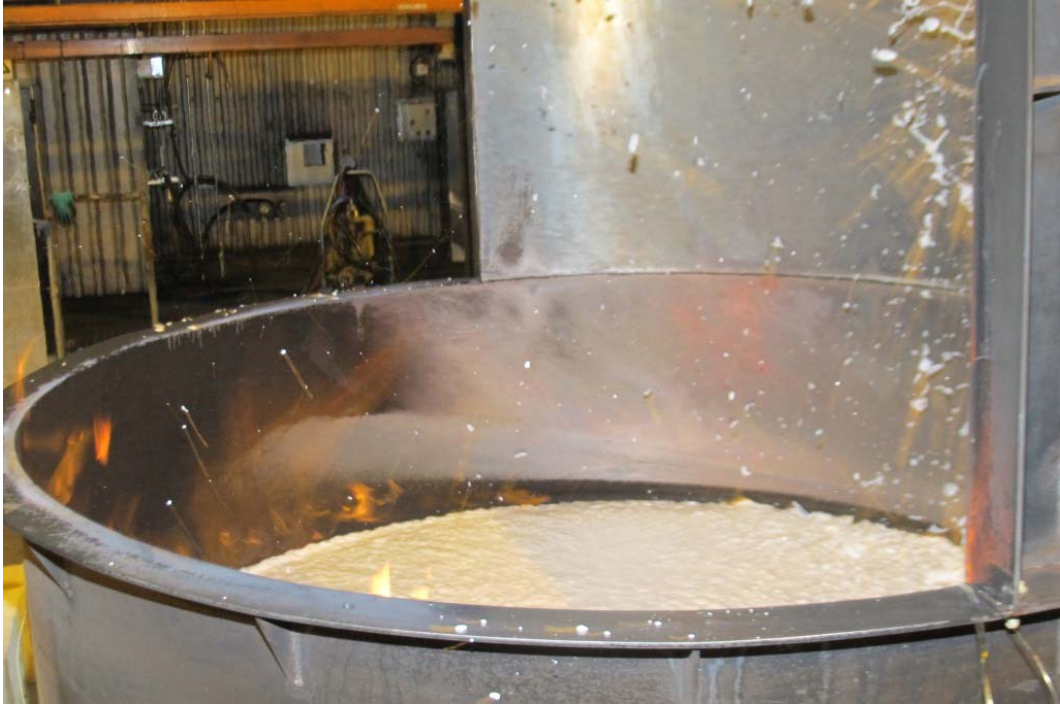
Figure 42 WP2-Test#2 (016) Using AFFF-AR at 6% concentration improved the fire extinguishing performance considerably.
