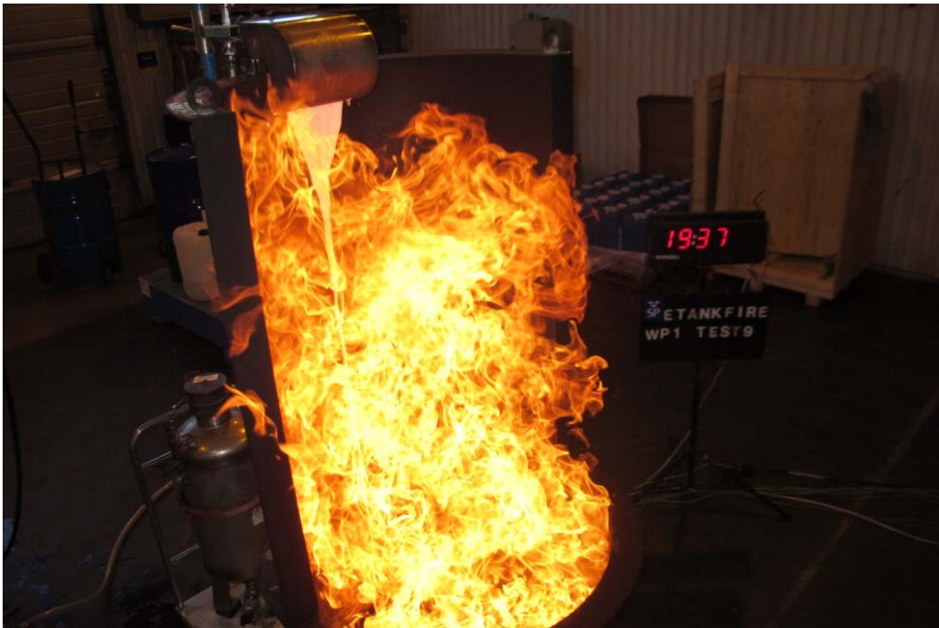
Figure 10 Test#9 (038) Foam chamber application, 1,55m above fuel surface. Still free fall of foam due to the hot steel wall (4:37 min:s after start of application).
