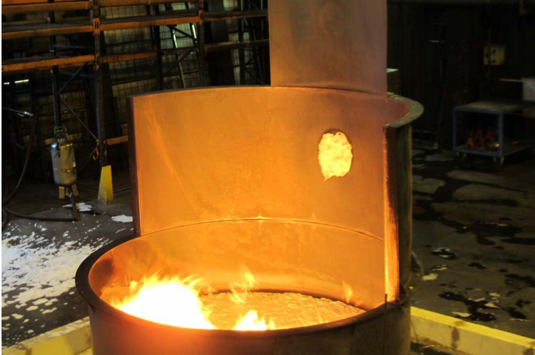
Figure 48 WP2-Test #8 (005) Similar to WP2-Test #1 (AFFF-AR 3%) but applied as CAF. Photo taken shortly after 8 min of foam application when we ran out of premix. The fire was extinguished manually.
