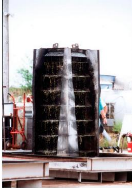
Figure C2 – NFPA18A fuel cascade.
