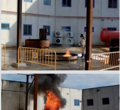
Top: the fire is in a standard test pan. The black, higherwalled pan in the background is the LASTFIRE test pan. Bottom: when the test is carried out using the LASTFIRE pan, the fire's characteristics are notably different. More heat is concentrated along the wall and the two baffles simulate possible obstacles that could be present in a real fire.
