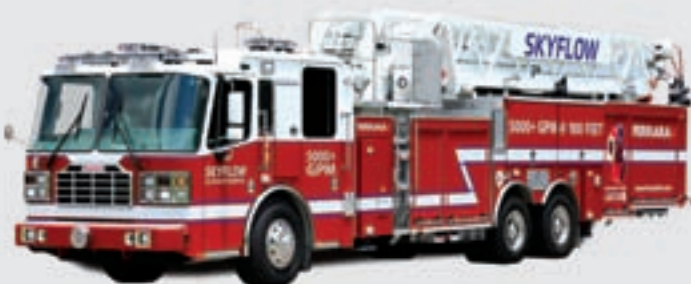
SKYFLOW SP-100 AERIAL 19,000+ LPM from aerial discharge 15,000+ LPM from dual rear monitors
