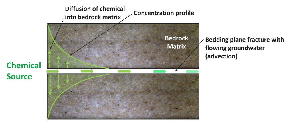
When a chemical source is introduced at an open, flowing bedrock fracture:
