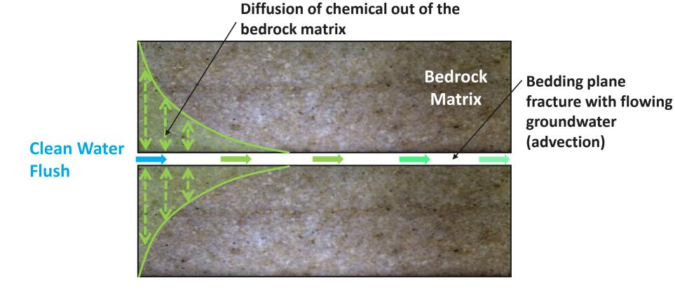
When a clean water flush (i.e. remediation) is attempted in a bedrock fracture:
