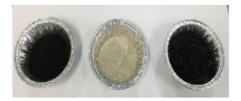
Adsorbents tested (left to right): aluminum hydroxide and carbon blend, clay, and pyrolyzed cellulose
