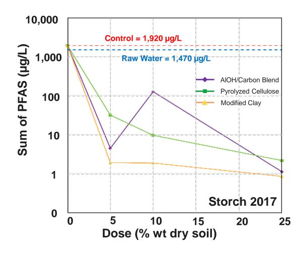
PFAS removal from supernatant in a soil/GW/adsorbent slurry at different % dry soil weight doses.
