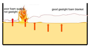
Picture 4: Extinguishing process of non film forming fluorine free foam type! No foam – no extinguishing!
