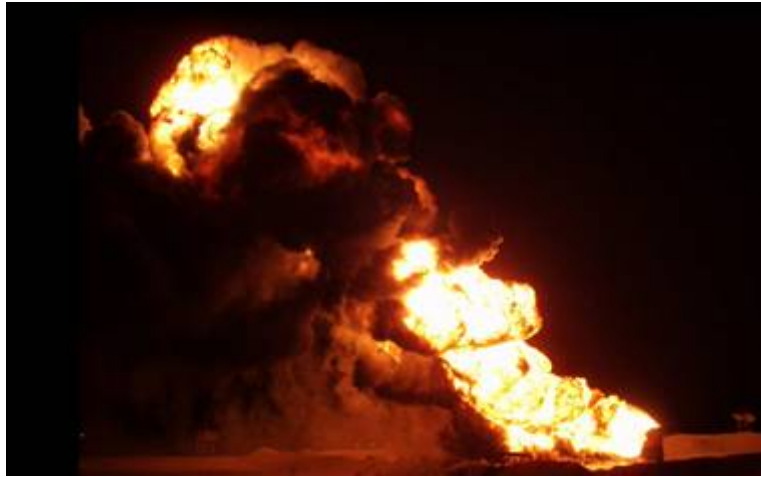
Flame from main boilover – estimated at 150m length (~6m diameter test pan)
