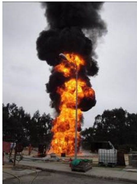
Typical boilover with 2.4m diameter test pan
