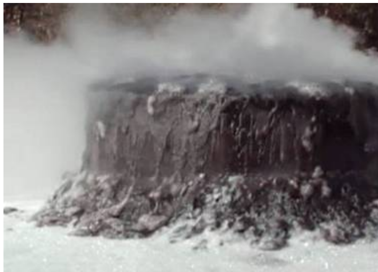
Fire extinguished but hot crude/foam emulsion continues to froth over from tank (2.4m pan)
