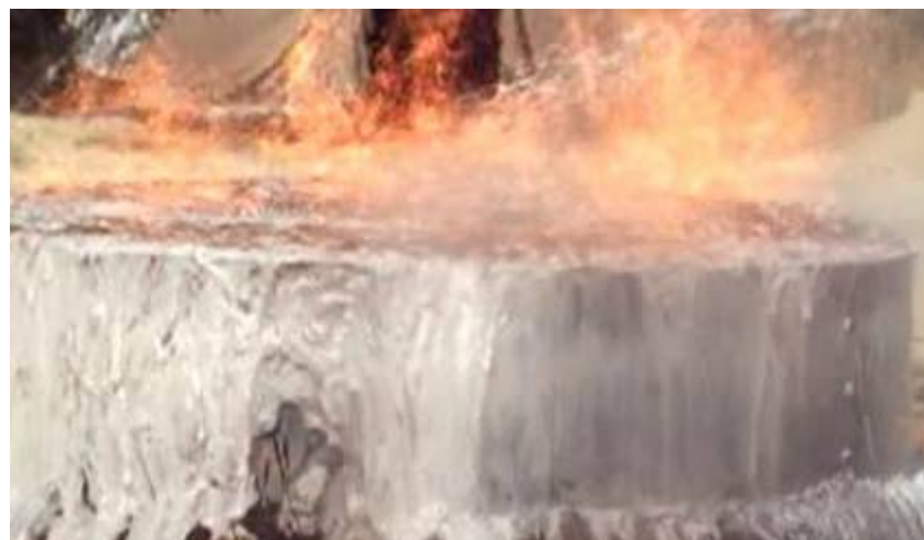
Sloper of burning fuel/foam during extinguishment attempt (2.4m pan)
