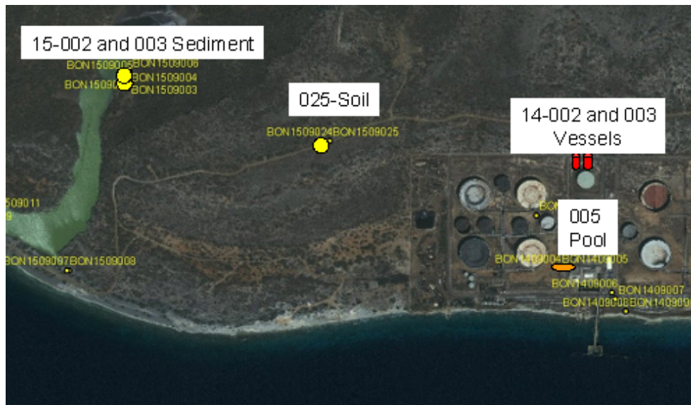
Figure 15 Detail of the map shown in Figure 14, showing the exact positions of the storage drums for the foams on the BOPEC area, the pool on the BOPEC area where fire fighting remnants were deposited as a sediment, and the nearest environmental sampling sites (1 soil and 2 sediment samples) outside the facilities. Other samples were taken at Lake Goto.
