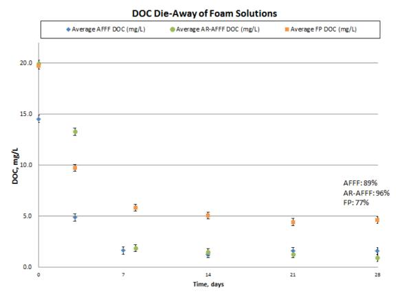
Figure 7: Foam degradation throughout DOC Die-Away testing
