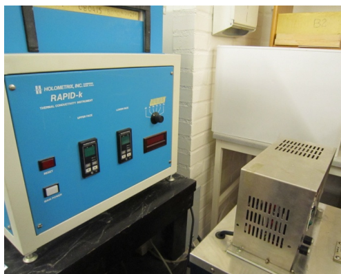
Figure 2.1: Holometrix Rapid-k apparatus, Chalmers University of Technology.
