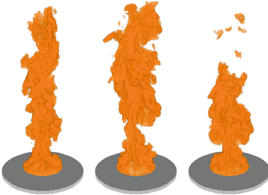
Fig. 32.4 Snapshots of the flame envelope from a simulation of the Sandia 1 m diameter methane pool fire using 1.5 cm grid resolution. The images span a single “puff”
