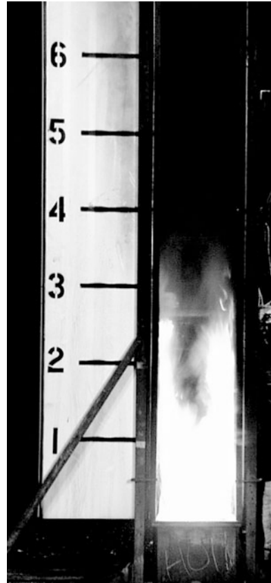
Fig. 36.17 Nonpropagating fire between two vertical parallel panels of a polymer (FPI < 6) for a test duration of 15 min [19]. The panels are about 0.61 m (2 ft) wide, 2.44 m (8 ft) high, and 25 mm (1 in) thick separated by 0.30 m (1 ft). The ignition source is a 60-kW, 0.30-m-wide, 0.61-m-long, and 0.30-m-high propane sand burner. The tip of the flame from the burner reaches a height of about 0.91 m (3 ft). Marks on the scale are in feet
