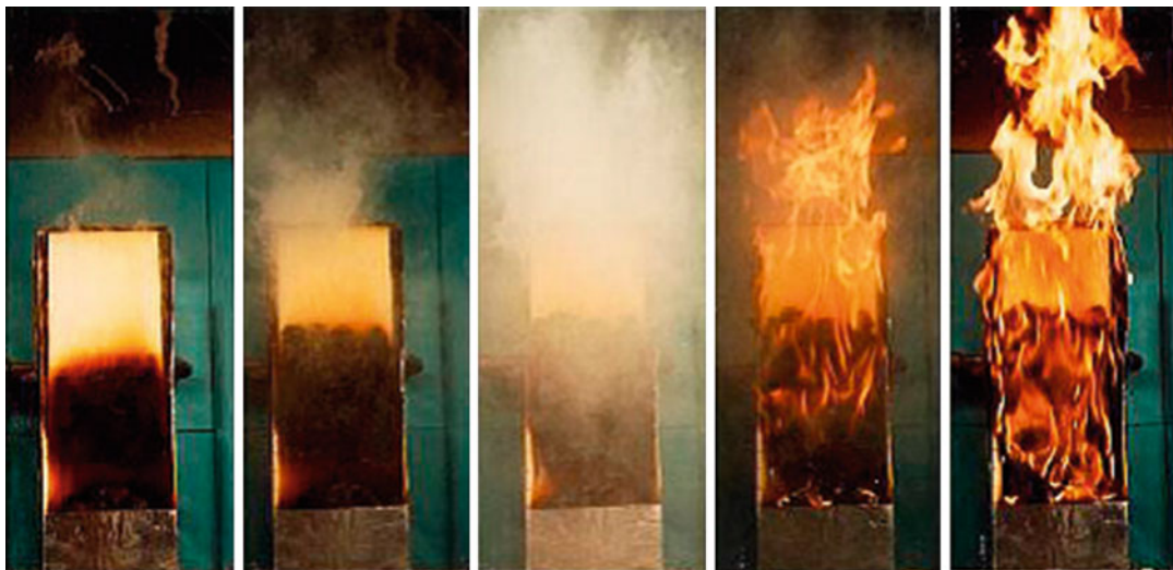
Fig. 19.14 Series of photographs of a combustion experiment illustrating the transition to flaming in a smoldering polyurethane slab 40 cm high under external forced flow (Photo by group of Prof. Carlos Fernandez-Pello, University of California at Berkeley). After 1 h of smoldering
