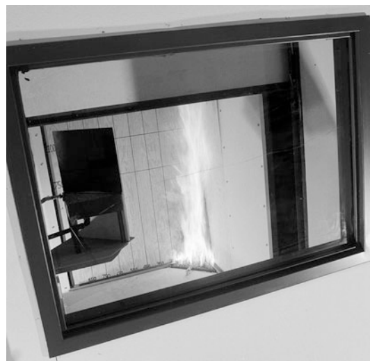
Fig. 27.19 SBI test in progress (Photo courtesy SwRI.)
