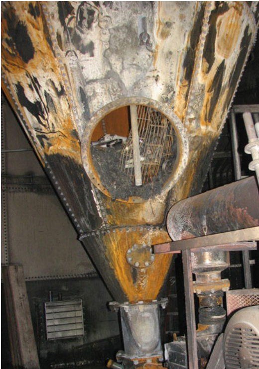
Fig. 70.11 Dust collector hopper in which coal dust explosion occurred
