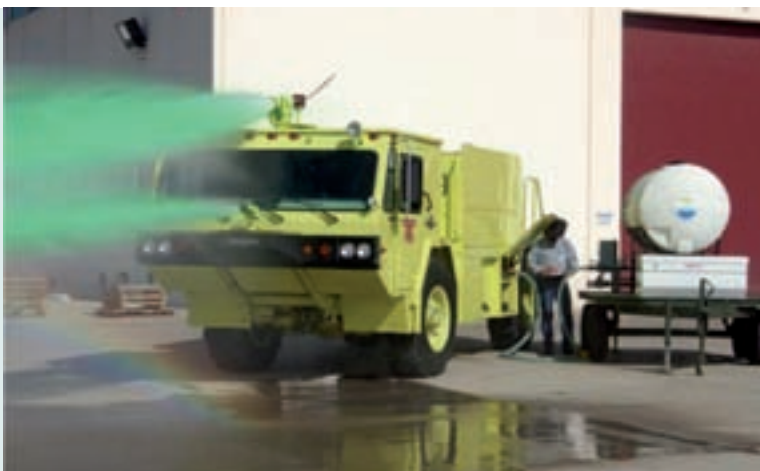
Top: bladder tank proportioning system set-up for surrogate liquid-type test. Below: ARFF vehicle being tested with water containing environmentally benign dye.
