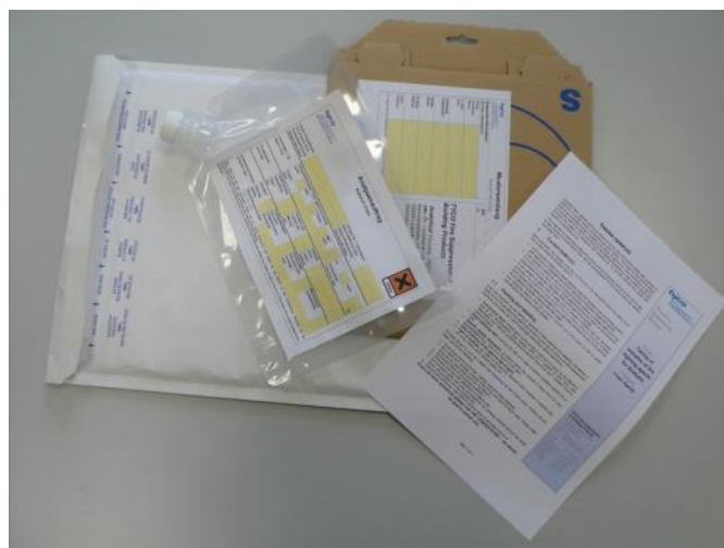
The PFOS sampling kit available from Tyco Fire Suppression & Building Products
