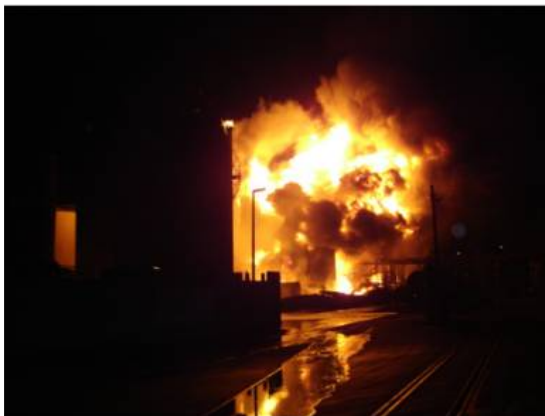
Figure 3. example of bund fire engulfing tanks situated in the bund
