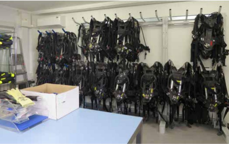
◀ Providing net cost reduction: Workshop for large scale SCBA cleaning, refilling and testing.
