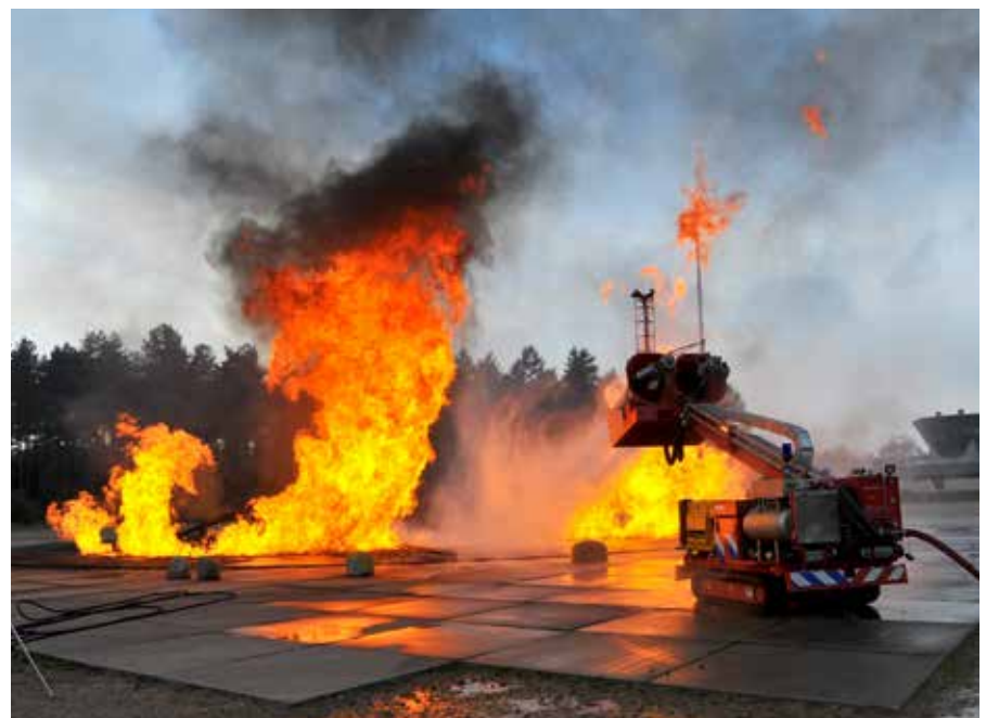
▼ Example of remotely operated firefighting robot.
