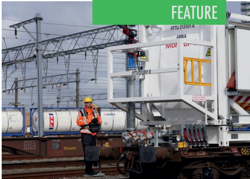
Remote controlled 4,000 L/min monitors are mounted on platforms at both ends of the train, handlines can be attached for manual foam application
