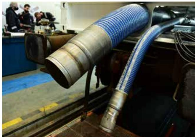
◀ Water system on wagons is connected with flexible hoses for track switches.
